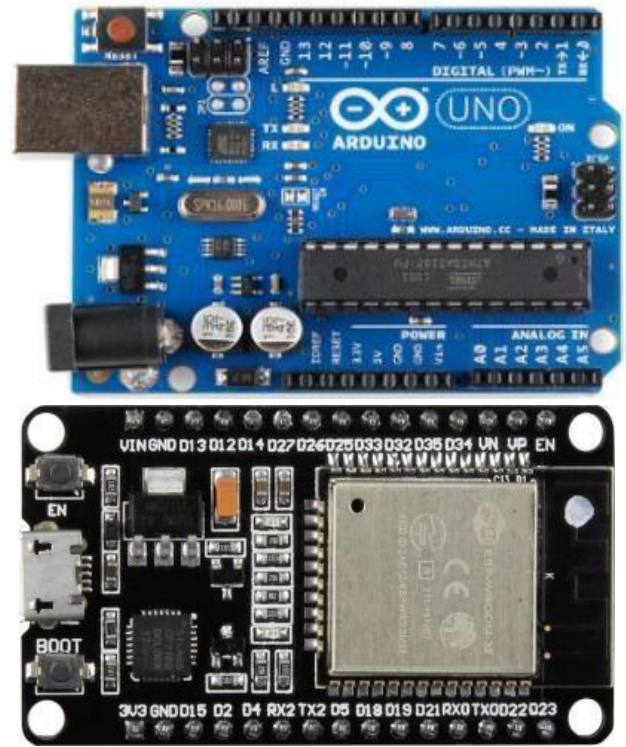
Figure 2.2: Examples of microcontroller units - Arduino Uno (left), ESP32 (right)
